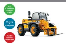
A versatile lifting machine that picks and carries materials. Lift loads from 4 mtr up to 20 mtrs.
