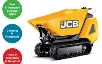
For moving building materials and aggregate. Narrow enough to fit through the average doorway for internal work, slip down side alleys or climb over steps and footings.
